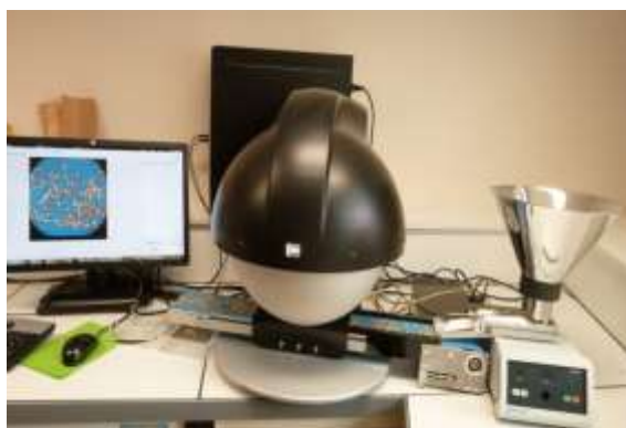
Figure 1 : Videometer et bande transporteuse (Videometer and conveyor belt)
