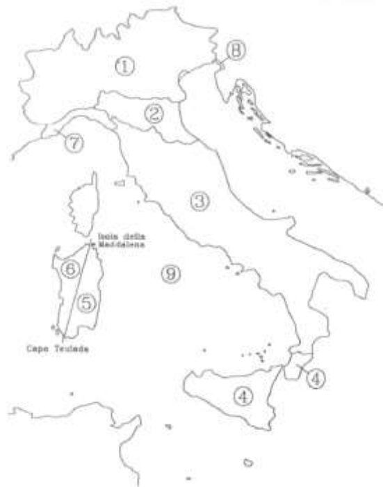
Figure 5 : Map of the nine different zones of Italy according to the reference wind speed of Eurocodice 1 (CNR, 2009).
