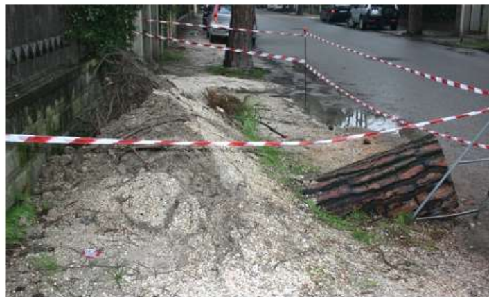
Figure 3 : Stump of Pinus pinea after failure with evident sinking of the base of the trunk in the compressed position compared to the fall direction.
